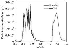
Fig.9 Spectral radiation of plume defined by threshold of 0.0005 and the standard one
