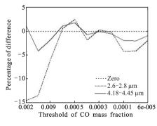
Fig.8 Percentage of differences of band radiation between plume defined by threshold of 0.0005 and the standard one
