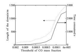
Fig.6 Length of plume domain and time consumed for calculation
