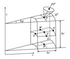
Fig.2 Schematic of control volume and control angle
