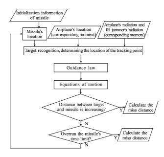
Fig.5 Simulation model of IR homing missile
