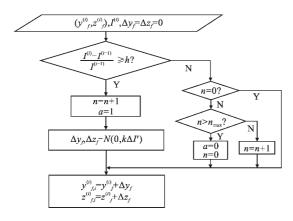
Fig.7 Simulation flow of cross-detector seeker's target recognition
