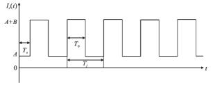
Fig.2 Waveform of jammer and target's superimposition signal
