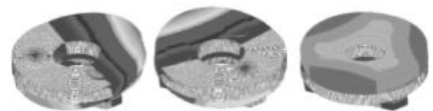
图 8 力学样机模态分析前三阶振型云图 Fig.8 First three modes of dummy PMA
