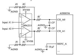
Fig.4 ADS8556 pre-conditioning circuit
