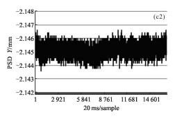
(c) Displacement fluctuation when light spot is around (2, 2) Fig.7 Experimental results of PSD displacement
