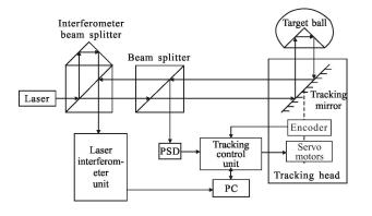
Fig.1 Laser tracking measurement system diagram
