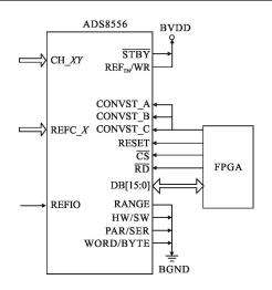
Fig.5 ADS8556 pin configuration
