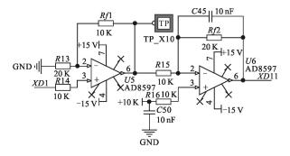
(b) Proportional difference operation circuit-X1Fig.3 PSD and its signal conditioning circuit
