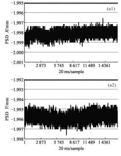
(a) Displacement fluctuation when light spot is around (-2, -2)
