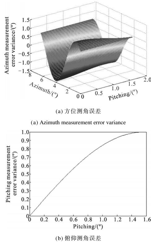
Fig.5 Angle measurement errors affected by sighting axis deviation
