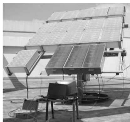
Fig.11 Test setup of non-tracking CPV module
