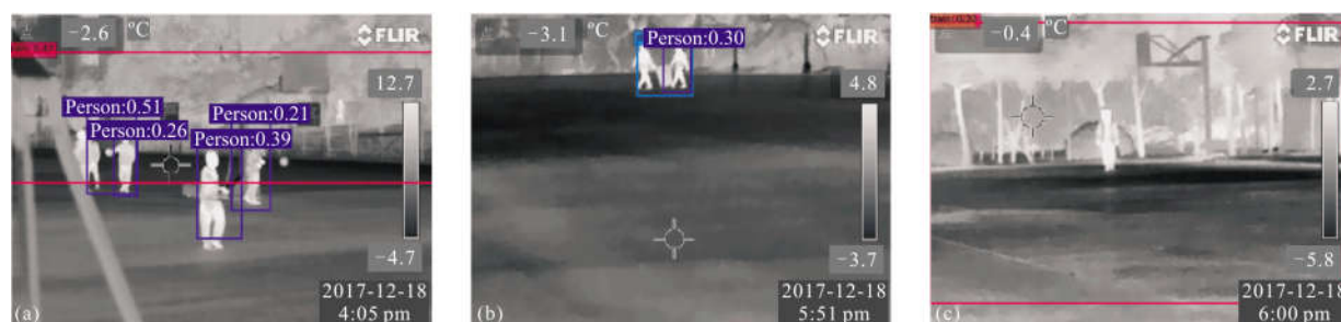
Fig.1 Infrared object detection with a visible object detection model (a), (b) and (c) represent three scenes
