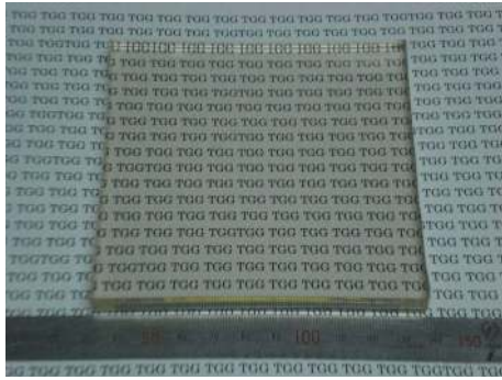
图 3 日本神岛化学制备的超过 10×10 cm 尺寸的 TGG 陶瓷 [42] Fig.3 TGG ceramic with a size over 10 cm×10 cm prepared by Konoshima Chemical, Japan [42]
