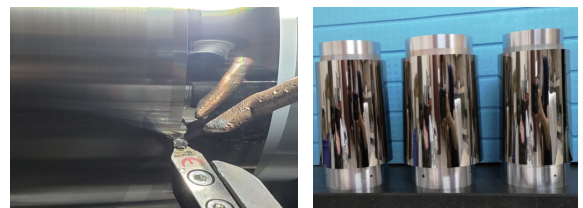
(a) 芯模超精车加工 (b) 超精车后的芯模 (a) Mandrel on ultra-precision turning (b) Mandrel after ultra-precision turning
