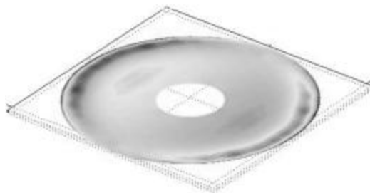
图 8 面形拟合结果 RMS=2.68\text{ nm} ( RMS=0.004\lambda , \lambda=632.8\text{ nm} ) Fig.8 Result of surface figure fitting RMS=2.68\text{ nm} ( RMS=0.004\lambda , \lambda=632.8\text{ nm} )
