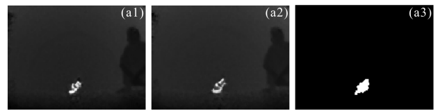
(a) 正庚烷火焰相邻帧深度图及识别图 (a) Consecutive depth maps and recognition image of n-heptane flame
