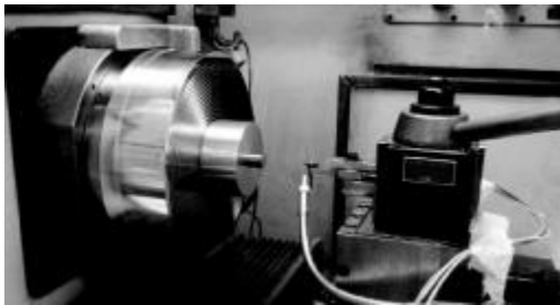
图 2 钛合金超精密切削实验 Fig.2 Ultra-precision cutting test of titanium alloy
