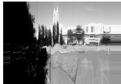
图 5 基于车载移动平台采集的原始高光谱线阵影像 Fig.5 Raw hyperspectral image is captured based on the mobile vehicle platform
