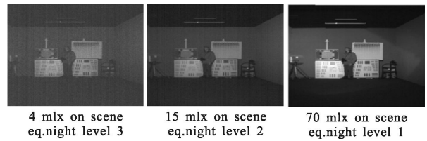
Fig.5 NOCTURN digital extreme low-light CMOS detector
