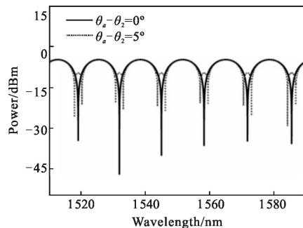
图5  $\theta_a-\theta_2$ 分别为0°和5°时的干涉谱Fig.5 Interference spectrum when  $\theta_a-\theta_2=0$  and 5° respectively
