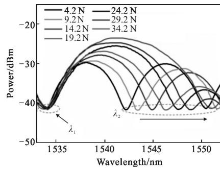
图 10 当  $\theta_a - \theta_2 \approx 0$  时,不同压力下的干涉谱Fig.10 Interference spectrum under different pressures when  $\theta_a - \theta_2 \approx 0$
