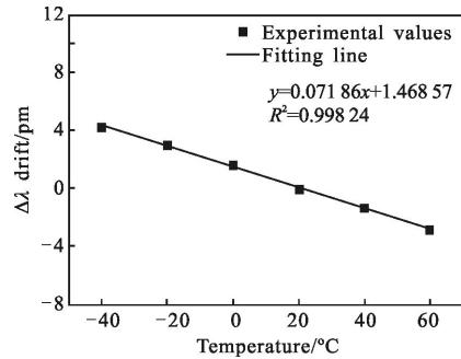
图 16 温度引起的波长差  $\Delta\lambda$  的漂移Fig.16 Wavelength difference drift  $\Delta\lambda$  due to temperature
