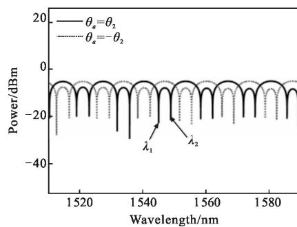
图4 当 $\theta_a+\theta_2=0$ 和 $\theta_a-\theta_2=0$ 时的仿真干涉谱Fig.4 Simulated interference spectrum when  $\theta_a+\theta_2=0$  and  $\theta_a-\theta_2=0$  respectively
