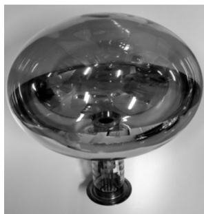
图 3 20 in MCP-PMT 实物图 Fig.3 Picture of 20 in MCP-PMT
