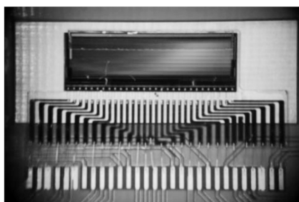
Fig.4 Microphotograph of the fabricated visible blind 640x8 pixel UVFPA
