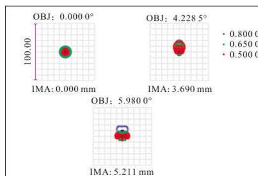
Units are  $\mu\text{m}$  Airy radius: 1.221  $\mu\text{m}$
