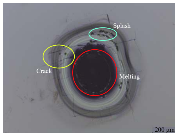
Fig.6 Metallographic structure of multi-effect coupling damage in monocrystalline silicon
