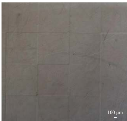
(a) PDMS 表面微结构 (光学显微镜) (a) Surface microstructure on PDMS (optical microscope)
