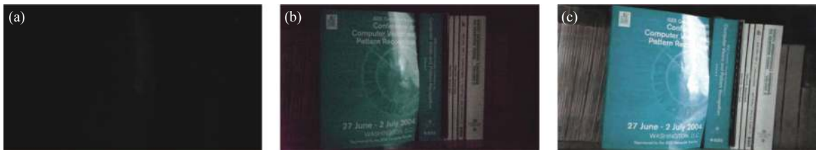
图 148 基于深度学习进行极弱光成像的结果。(a) 摄像机输出 (ISO 8000); (b) 摄像机输出 (ISO 409600); (c) 由原始数据 (a) 恢复得到的结果 [705] Fig.148 Results of extremely weak light imaging based on deep learning. (a) Camera output with ISO 8000; (b) Camera output with ISO 409600; (c) Our result from the raw data of (a) [705]
