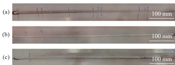
图 8 焊缝渗透探伤。(a) 未处理; (b) 人工打磨后; (c) 激光清洗后 Fig.8 Weld penetration inspection. (a) Untreated; (b) After manual grinding; (c) After laser cleaning
