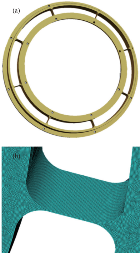
图 10 (a) 优化后的像旋补偿机构; (b) 像旋补偿机构有限元模型 Fig.10 (a) Optimized image rotation compensation mechanism; (b) Finite element model of image rotation compensation mechanism
